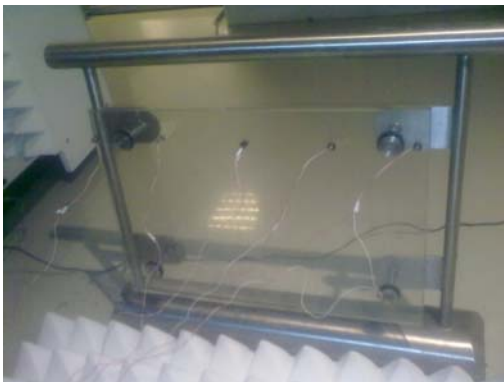
Fig.1. The transducer mounted on the one-layer glass with a digital amplifier (top) and fixing of the glass for the vibration measurements (bottom).
