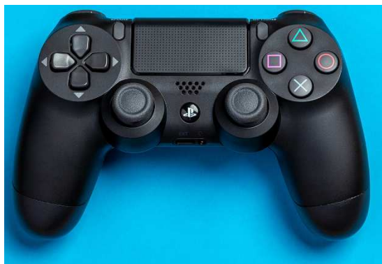
Fig. 2. Classic design for a game controller used for PS4. Ergonomic design helps two-handed handling. Some controllers have integrated tablet holders or steering wheel and pedal extensions.
