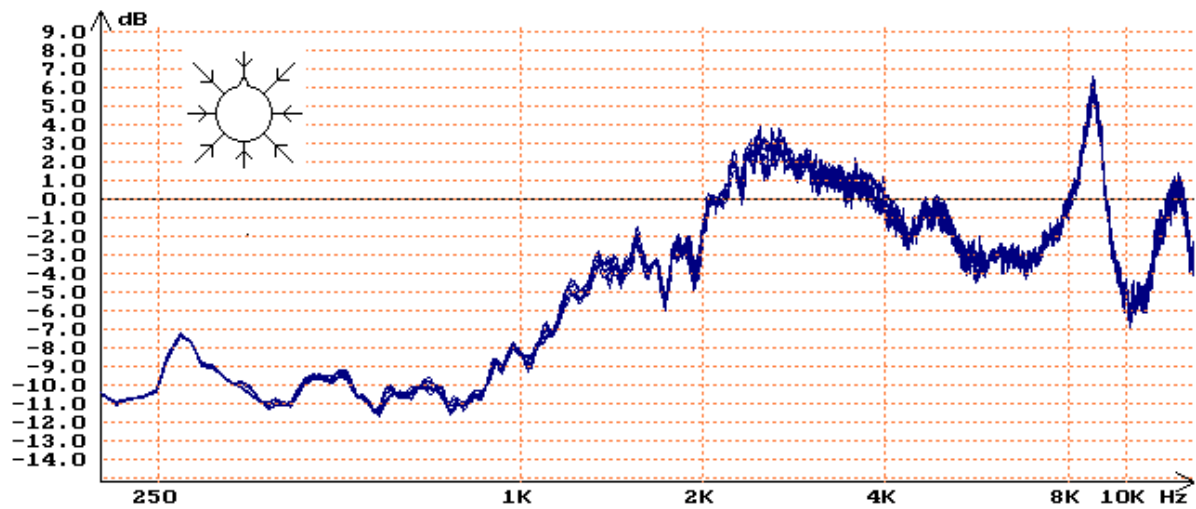
Fig.36. Testing the elevational settings. Set of HRTFs measured in 45° azimuthal steps (9 HRTFs, left ear).
