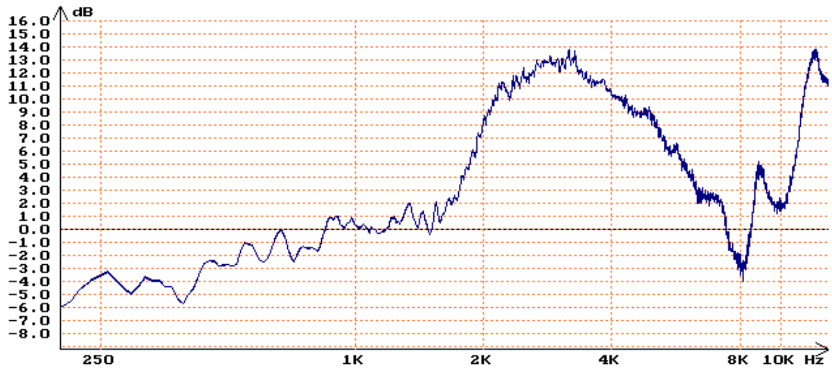
Fig.45. HRTF measurements by averaging of 768 and 15840 frames in the direction \delta=\varphi=0^\circ (left ear). These correspond to an increase of the SNR of +28,85 dB and +42 dB respectively. There is no visible difference.
