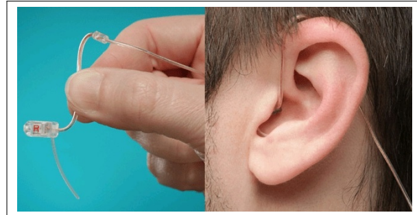
Figure 3. The tube-like EarHero Pro model without the soft bud (left) and inserted at the entrance of the partly open ear canal (right).
