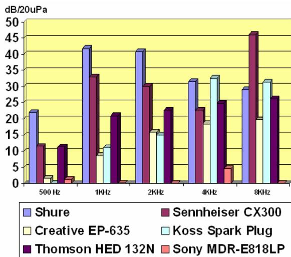
Figure 8. Sound isolation of six earphones at various frequencies at frontal incidence.
