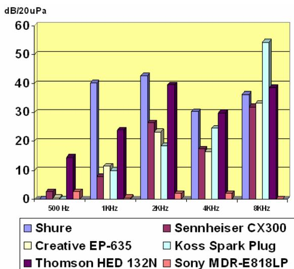
Figure 9. Sound isolation of six earphones at various frequencies at lateral incidence.
