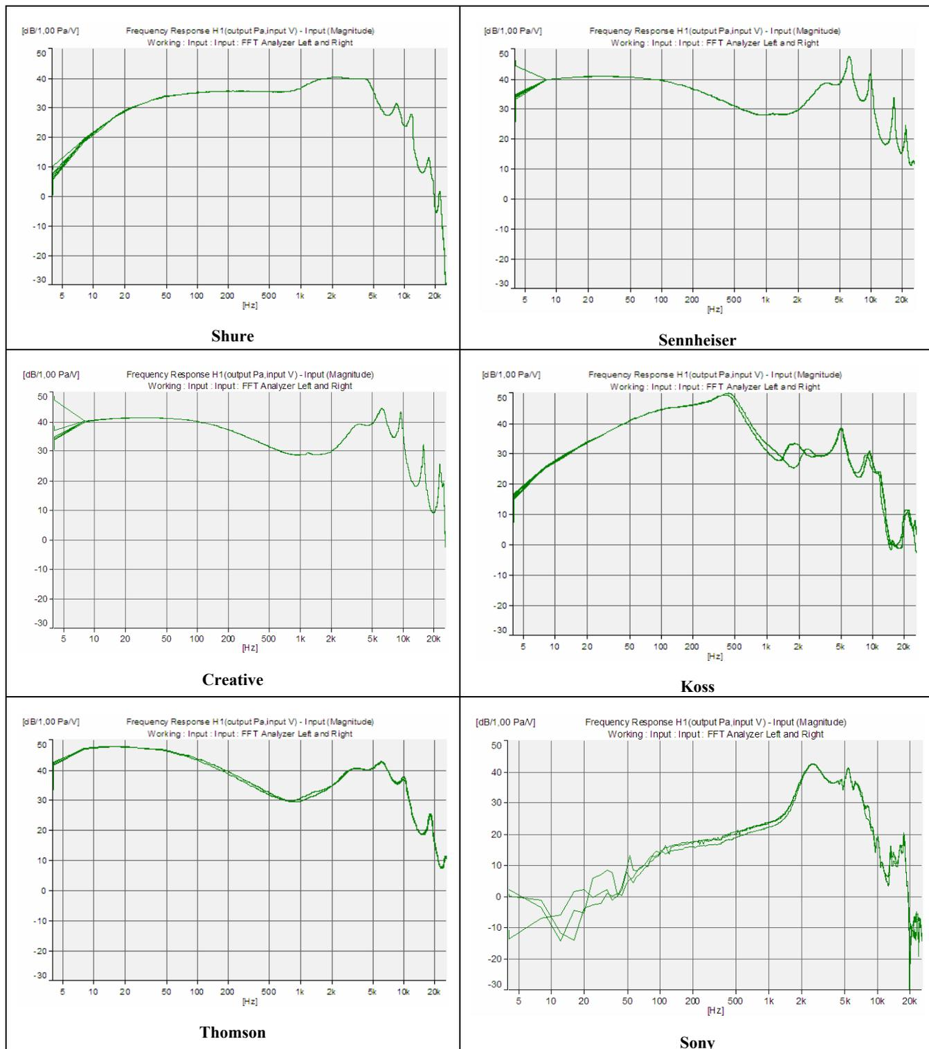
Figure 7. Transfer function measurements of six earphones.
