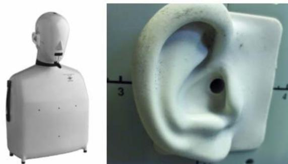
**Figure 2.** The BK4128 dummy-head and the DZ 9629 pinnae. Note the relatively small diameter of the (non-blocked) ear canal entrance.
