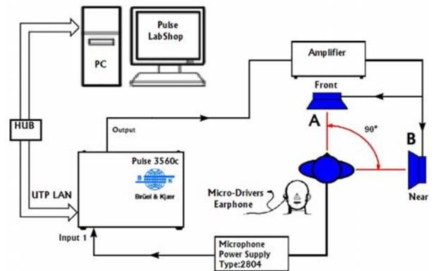
**Figure 6.** The measurement setup for sound isolation measurements.
