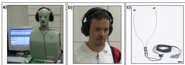
Figure 7. The BK 4128 dummy-head (left), individual measurements (middle) and the BK 4101 binaural microphone (right).
