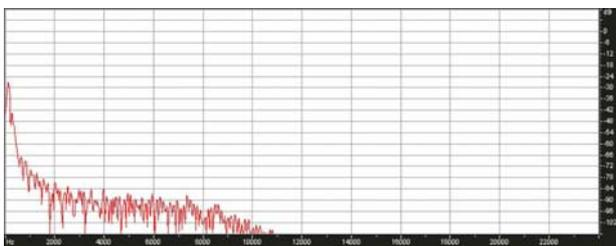
Figure 3. Spectral representation of the word "print" (in Hungarian). Compressed spearcon based on a text-to-speech application.
