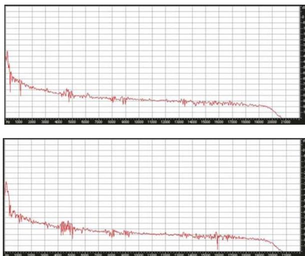
Figure 1. Spectral representation of the word “print” (in Hungarian). Original recording (top) and compressed spearcon (bottom) in 16 bits, 44100 Hz resolution.
