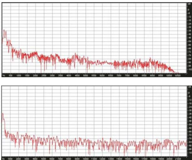
Figure 2. Spectral representation of the word "print" (in Hungarian). Compressed spearcon in 16 bits, 22050 Hz resolution (top) and in 8 bits, 44100 Hz resolution (bottom). Compare it with Figure 1.
