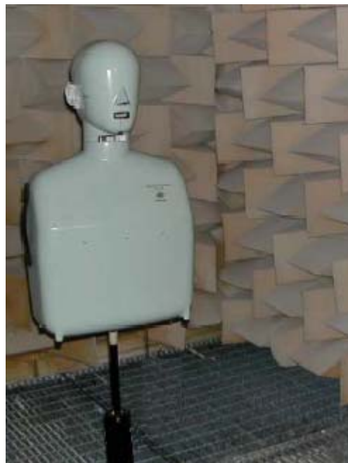
Fig.2. The Brüel & Kjær Head and Torso Simulator Type 4128 in an anechoic chamber.
