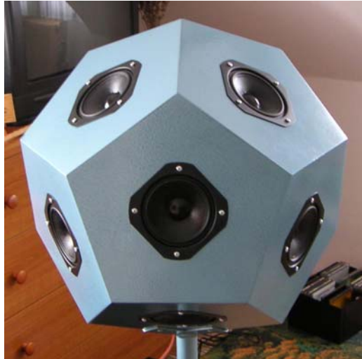
Fig.3. Omni-directional loudspeaker for measurements built by a student.
